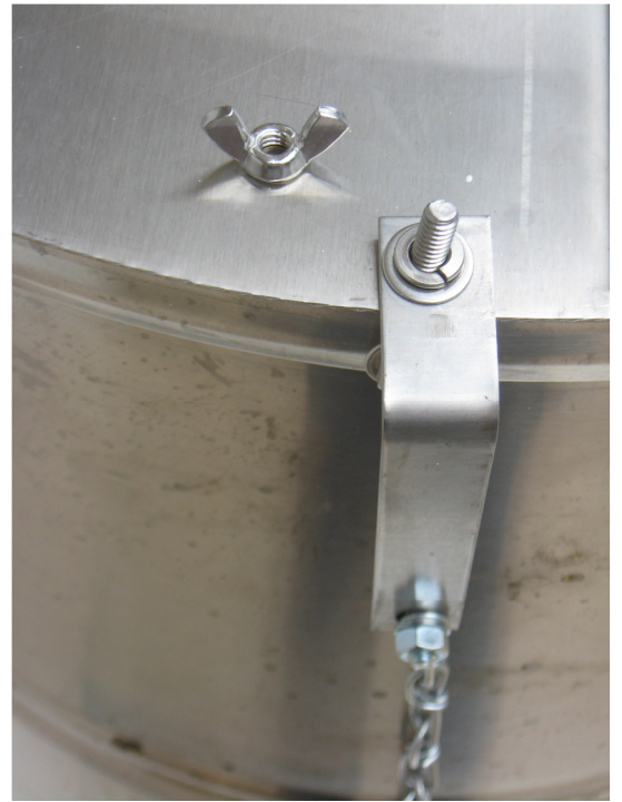
Figure 5 – Chain assembly with washers hanging over “L”-bolt.
