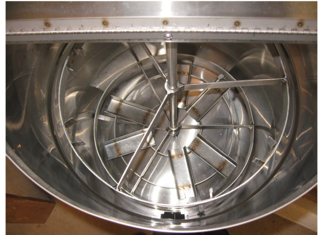
Figure 7 – Radial Reel in tank Note frame brackets on lower and upper rings. Frame top bar is placed toward edge of tank.
