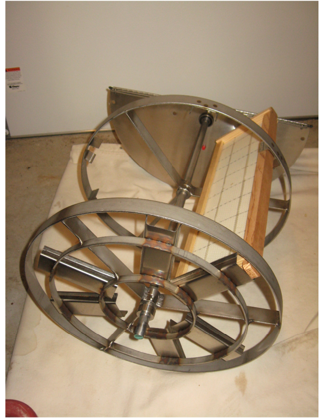
Figure 2- Radial Reel Bottom shaft end mates to nylon bushing at bottom of tank. NOTE FRAME PLACEMENT: Frame sides set in trays on bottom, top bar to the outside of the tank with frame 'ear' hanging over edge of the frame tray.
