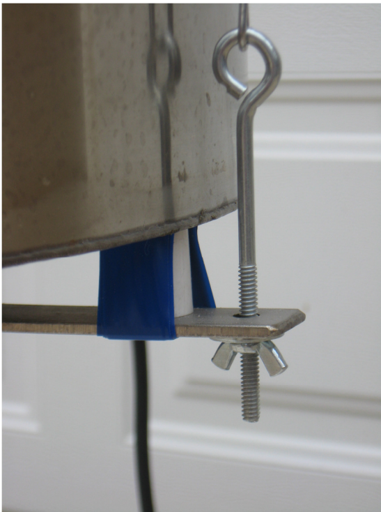
Figure 6 - Chain Assembly secures Tank to Stand.
